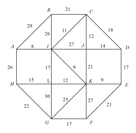
(a) Show clearly on the network the minimum solution to connect each wireless access point to form complete coverage. [3]
